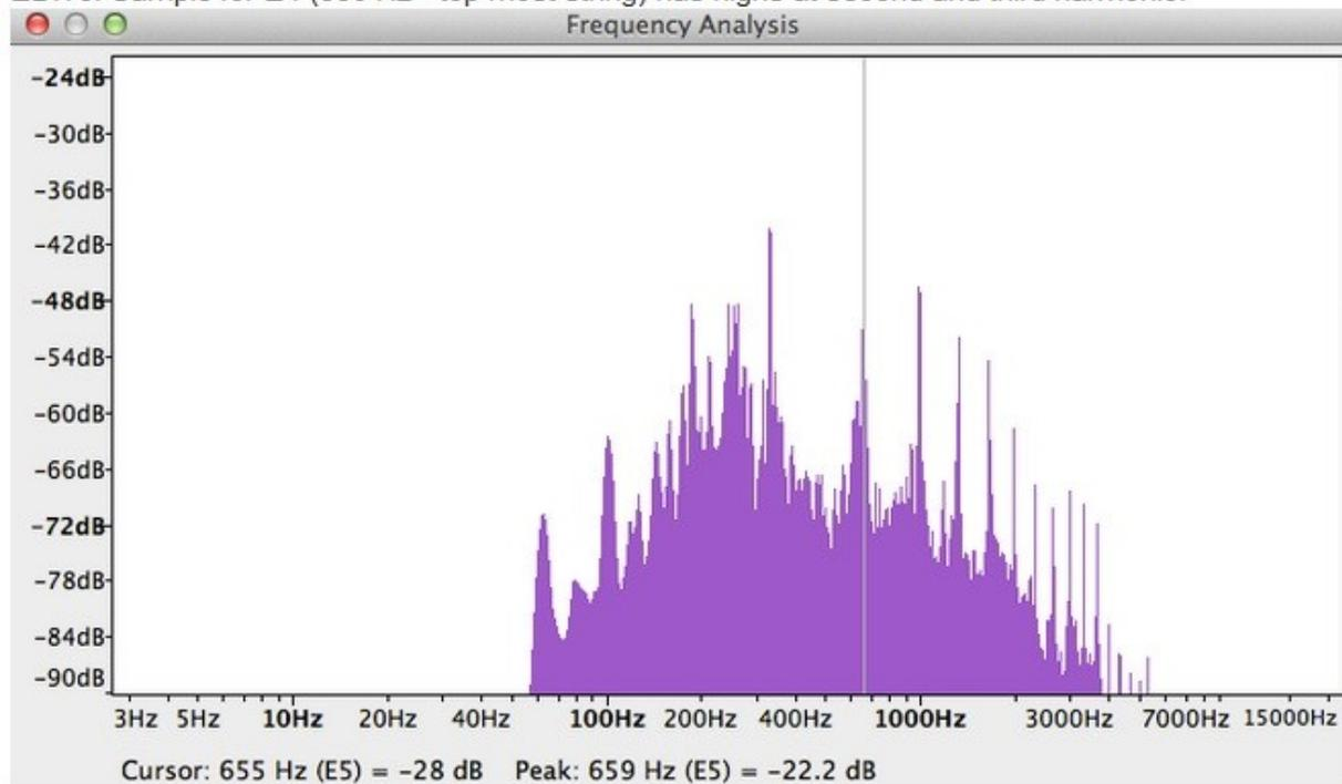
Figure 1 – Harmonic Spectrum of a Vibrating String
