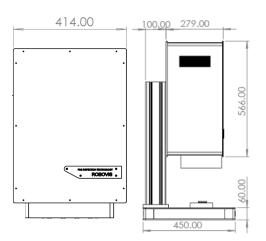
\*Vision head dimensions are the same in Inline and Desktop Versions (Size of the Vision Head can be adapted for specific requirements).
