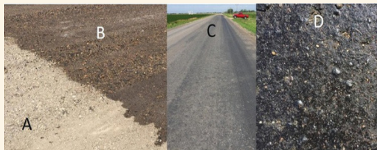
A) Untreated gravel. B) 30 minutes after treatment. C) After 6 weeks D) Close up of treated road surface. (Actual test conducted on gravel with a 25% asphalt regrind mixture).
