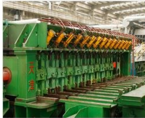
Three-roller Sizing Line With 14 Machines
