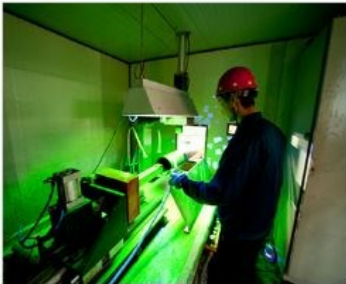
MPI for pipe ends
