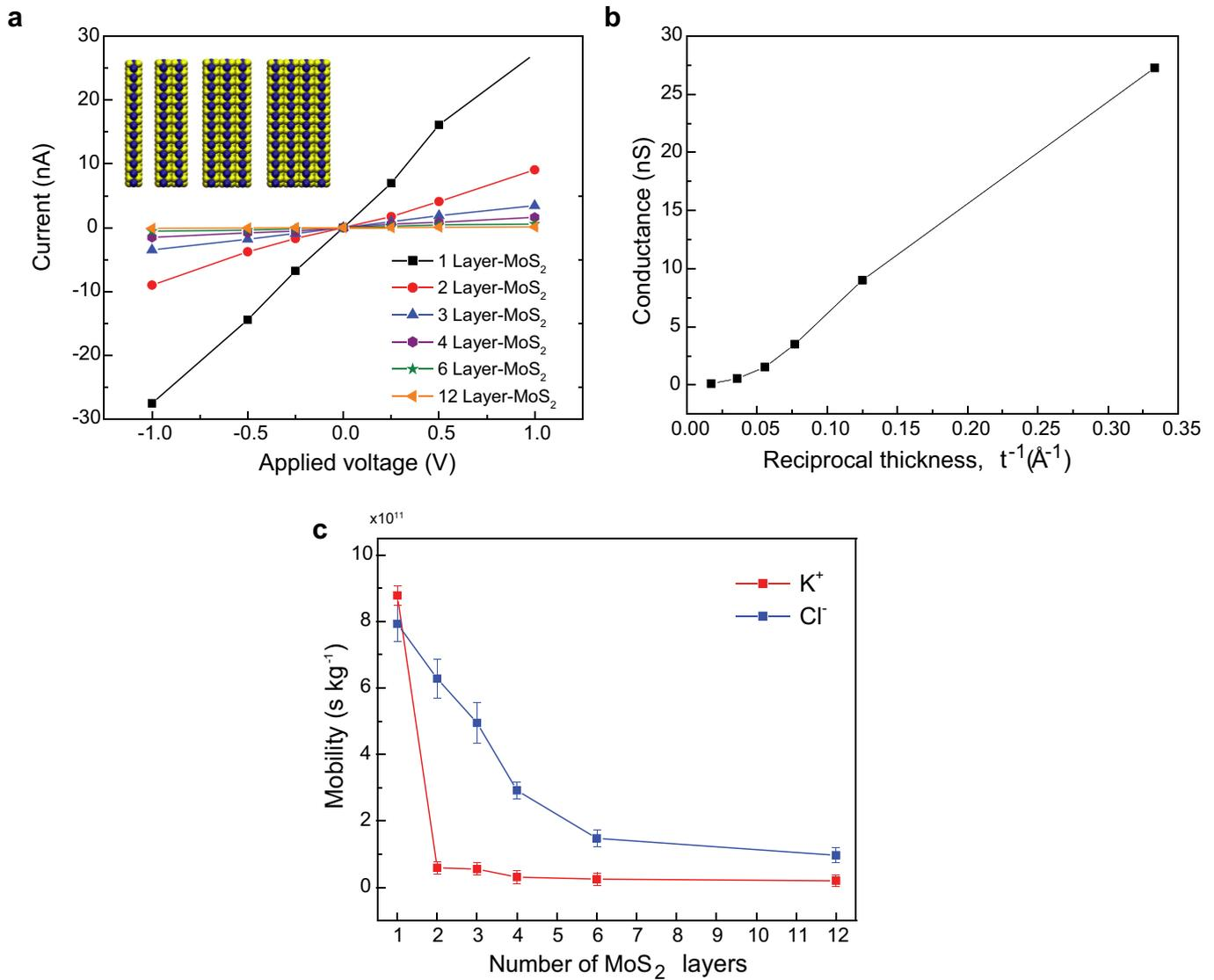
**Extended Data Figure 6 | Molecular-dynamics-modelled conductance as a function of membrane thickness.** a,  $I$ - $V$  curves for six membranes with a different number of MoS<sub>2</sub> layers, across a symmetrical 1 M KCl solution. The inset illustrates simulated multilayer membranes.
