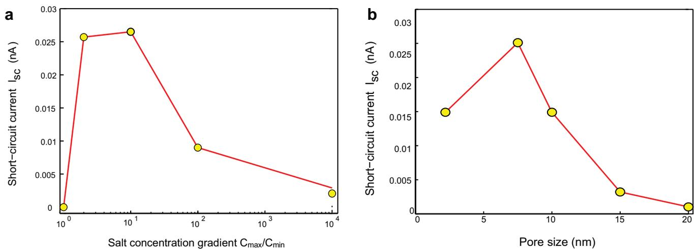
**Extended Data Figure 5 | Continuum-based PNP modelling of power generation.** **a**, Short-circuit current,  $I_{sc}$ , as a function of the concentration gradient ratio. The diameter of the nanopore here is 2.2 nm. **b**,  $I_{sc}$  as a function of the nanopore diameter. The salinity concentration ratio is fixed at 1,000. The surface charge of the nanopore,  $\sigma_n$ , is  $-0.04694 \text{ C m}^{-2}$ .
