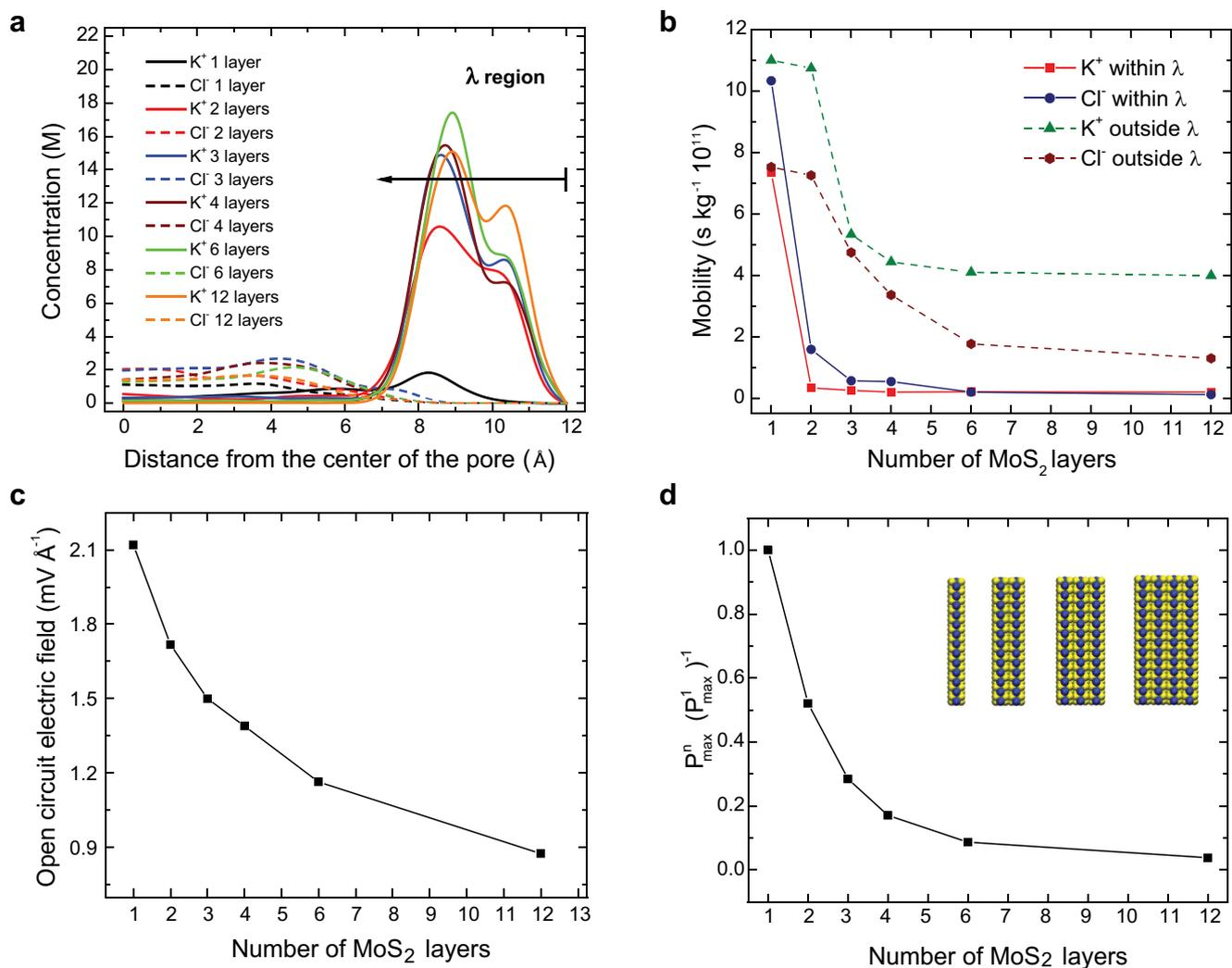
**Extended Data Figure 7 | Simulated power generation as a function of membrane thickness.** **a**, K<sup>+</sup> and Cl<sup>-</sup> concentrations as a function of the radial distance from the centre of the pore for single-layer and multilayer membranes. The  $\lambda$  region, near the charged wall of the pore, is representative of the electrical double layer. **b**, The mobility of each
