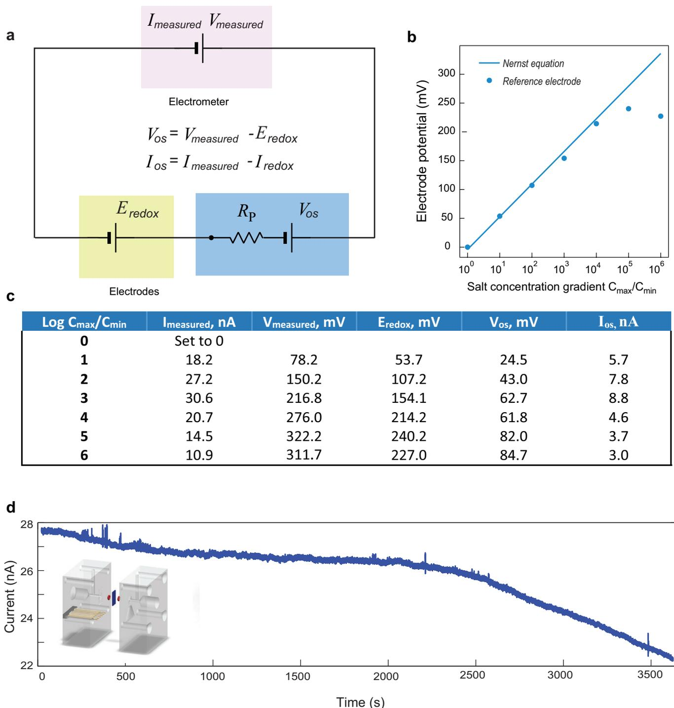
**Extended Data Figure 1 | Subtraction of the contribution made by electrodes, and stability of the nanopore generator.** **a**, Diagram showing the contributions of different parts of the system to the overall measured current. The osmotic contribution is obtained by subtracting the contribution of the potential difference at the electrodes from the measured voltage or current.  $V_{measured}$  is the measured voltage;  $E_{redox}$  is the
