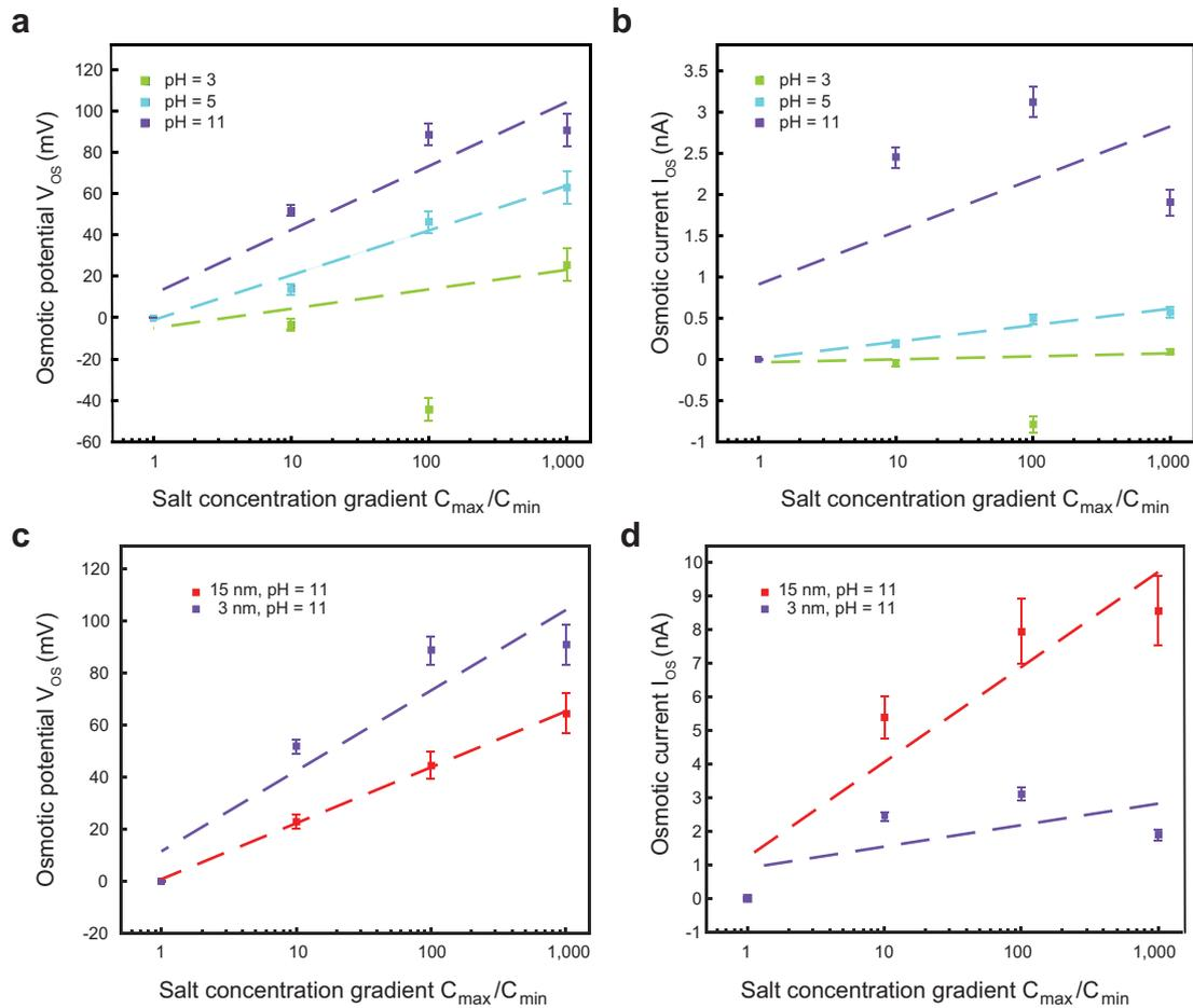
**Extended Data Figure 2 | Dependence of osmotic power generation on pH and pore size.** **a, b**, Osmotic potential (**a**) and osmotic current (**b**) generated using a 3-nm pore under different pH conditions (pH 3, 5 or 11) and in different concentration gradients. Power generation (both osmotic potential and osmotic current) at pH 3 is very low and sometimes
