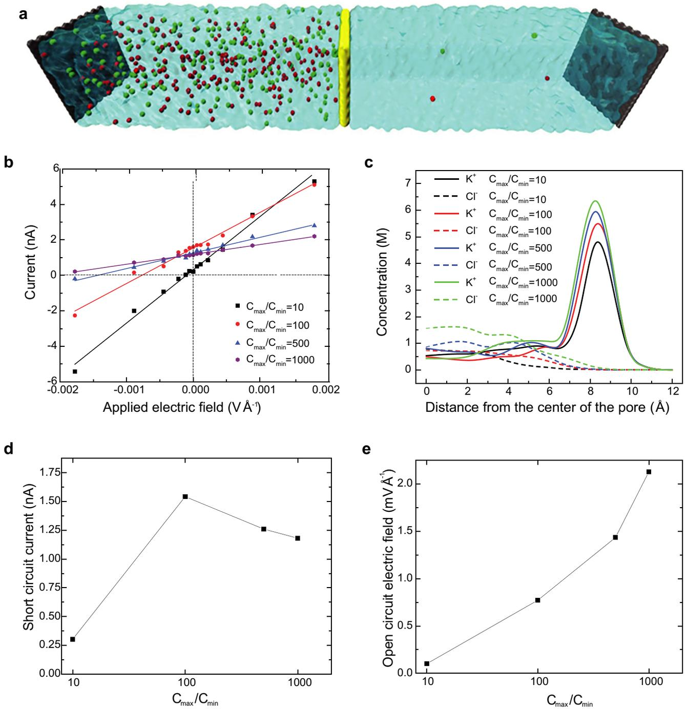
**Extended Data Figure 4 | Molecular-dynamics simulations of power generation for various ratios of concentration gradients.** **a**, A typical simulation box. **b**, Current as a function of the applied electric field for a single-layer MoS<sub>2</sub>, at different concentration ratios. **c**, K<sup>+</sup> and Cl<sup>-</sup>
