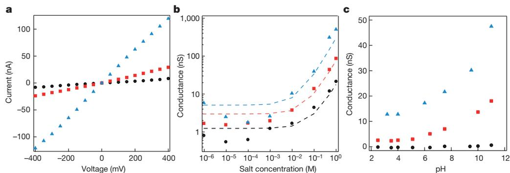
**Figure 2 | Electrical conductance and chemical reactivity of the MoS<sub>2</sub> nanopore.** **a**, Current–voltage response of MoS<sub>2</sub> nanopores with different pore sizes (black, 2 nm; red, 6 nm; blue, 25 nm) in 1 M KCl at pH 5. **b**, Conductance as a function of salt concentration at pH 5. By fitting the
