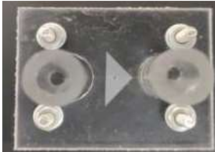
Device 1: Micro-Nano Fluidic Chip, MM scale fluid storage
