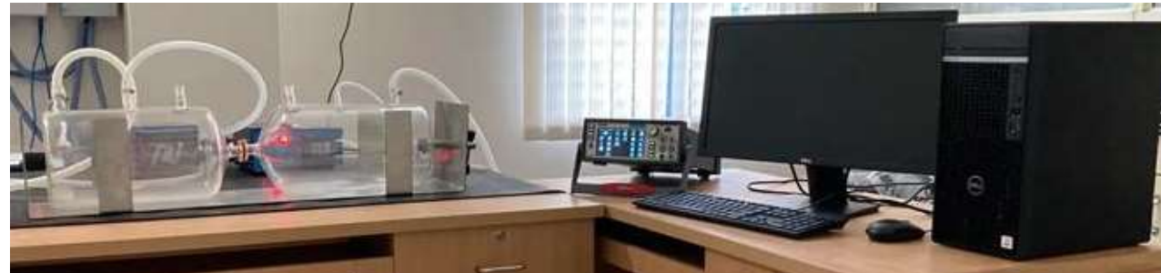
Device 2: MM/cm scale Osmotic Power Generator, large cm scale fluid storage
