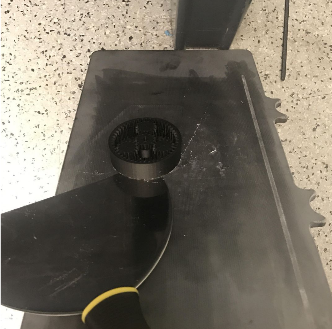
Figure 3. Removal technique for getting the part off of the build plate using a paint scraper.
