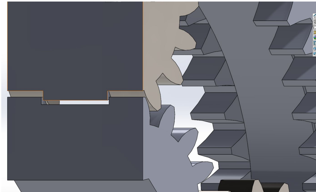
Figure 5: Gap of .025" between flat tooth faces
