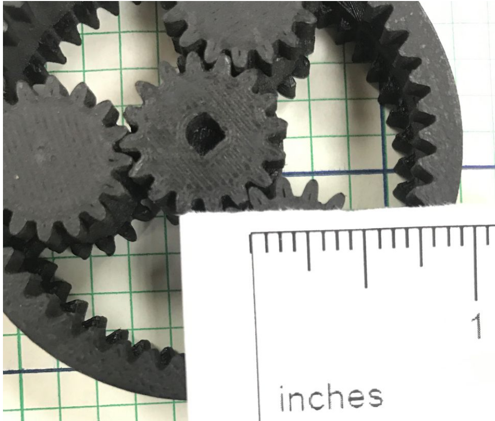
Figure 3. Image showing delamination issues observed in gear teeth.
