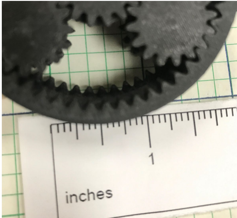
Figure 1. Image showing overhangs on printed part.
