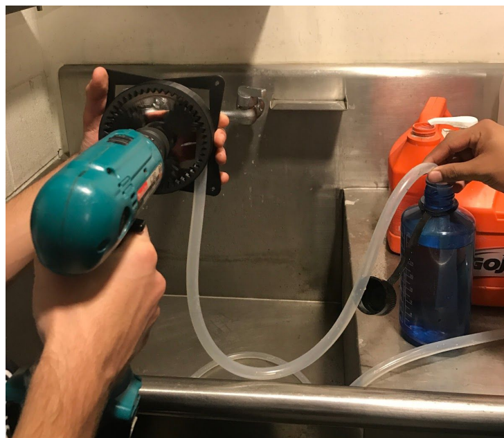
Figure 5. Image of testing performed to determine functionality when pumping water.
