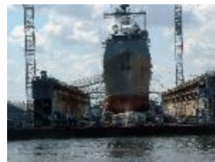
Ship Sitting in a floating "Dry Dock" For Repairs
