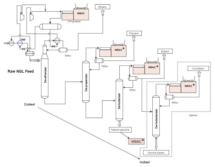
\*Note: These WSAC streams are combined into a common unit with separate bundles.
