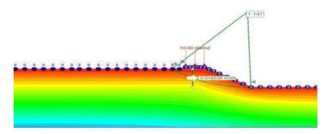
Fig 7 FOS for dynamic seepage analysis of starter dyke
