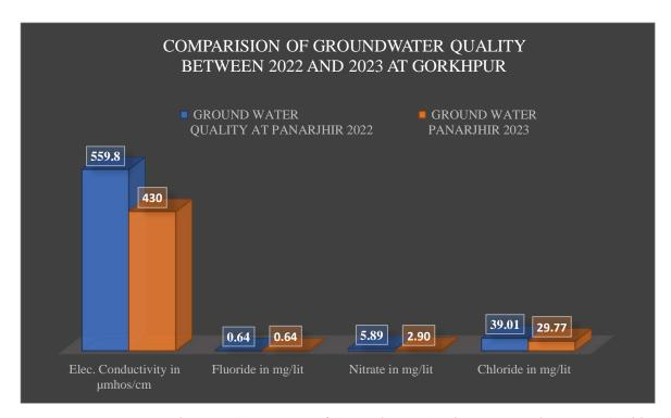
Figure-22: Histogram showing Comparison of Groundwater Quality (2022 and 2023) at Gorkhpur.
