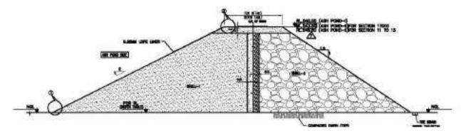
Fig 2 Cross Section of starter dyke
