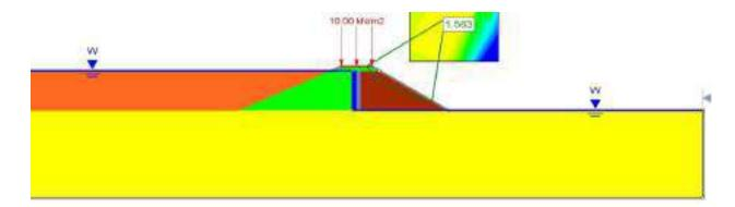
Fig 5 FOS for static analysis of starter dyke
