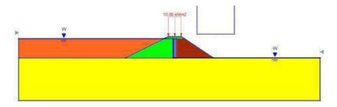
Fig 3 Model for static analysis of starter dyke
