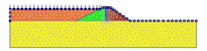
Fig 4 Model for seepage analysis of starter dyke
