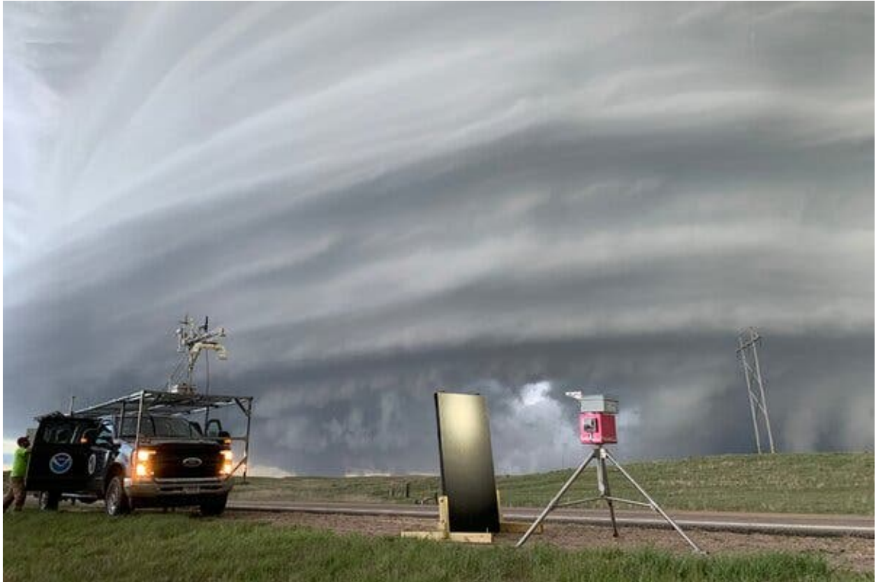
Weather research equipment with the Targeted Observation by Radars and UAS of Supercells project of the National Oceanic and Atmospheric Administration, including a “hail camera” in the front of the truck, in Nebraska. Credit...Sean Waugh/NOAA
