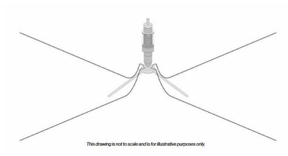
The manual notes that adding more radials, going from 4 to 16, will offer an increase of about 1.5dB. This is actually not the same as gain when you add a parasitic element to a horizontal dipole and achieve gain over the dipole (which is due to re-distributing the energy emitted by the dipole). The noted 1.5dB is from reducing the ground loss through adding more radials.
