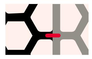
Dowel pins are often used when two or more panels are to be placed next to each other that have continuous artwork without a border. These pins give great stability to the panels. Here are some things to keep into consideration:
