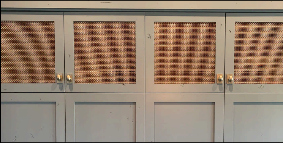
Wire Mesh, Designer Mesh, SHIRE™ 8148, Copper/Stainless Steel, Copper Alloy/Type 304, Woven - storage cabinet. Flat Warp/Round Fill Weave, 41% Open Area provides a stylish accent as infill panels in this custom built
