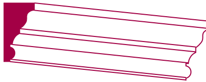
No. 507 Fancy Molding Height: 4 1/2" Projection: 3 1/2"
