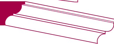
No. 525 Molding Height: 3 3/4" Projection: 4"
