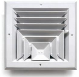
Made of aluminum and available in 4 sizes, the Square Ceiling Diffuser 3-Way is the visible part of the air conditioning system that is mounted in the ceiling of a residential or commercial building. With a **270°** air diffusion pattern, this multi-louver model distributes air flow throughout the room and includes a damper for flow control as well as 4 screw holes for mounting / installation.
