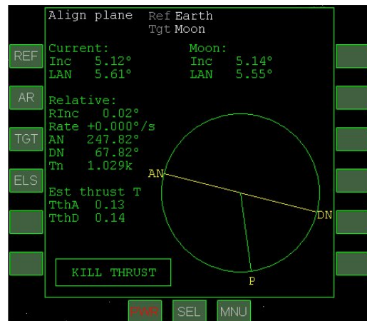
After normal (-) burn, RInc reduced to 0.02° for accurate use of Transfer MFD
