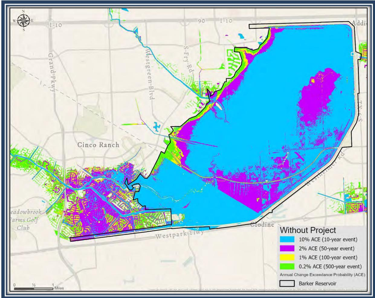
Figure 15. Barker Dam and Reservoir Map Showing the 2020 0.1, 0.02, 0.01, and 0.002 AEP
