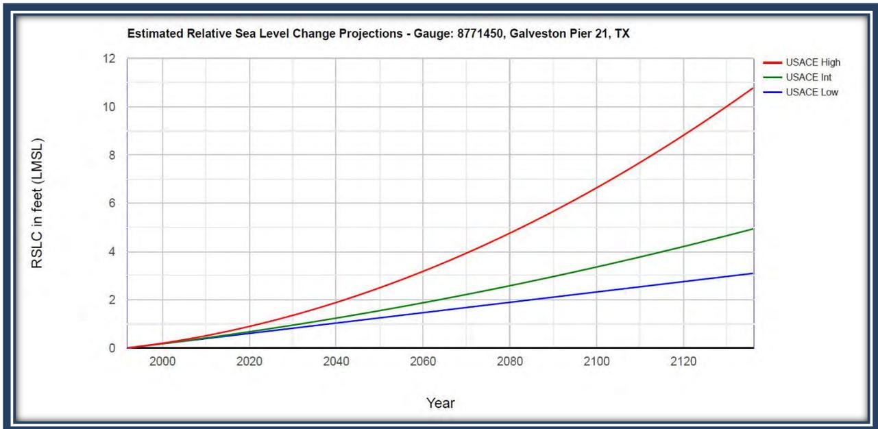
**Figure 25. Graph Showing Possible Relative Sea Level Change at Galveston's Pier 21**
