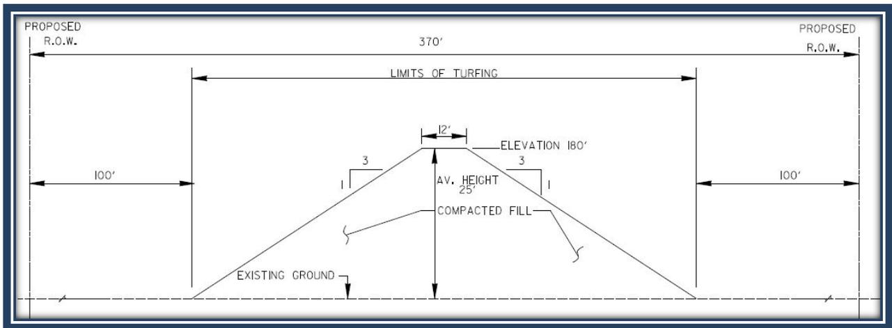
**Figure 32. Typical Embankment Section (Res2c)**
