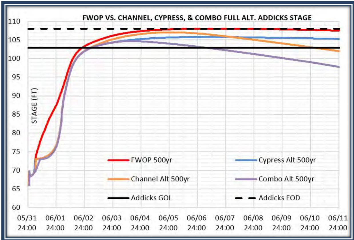
Figure 3. Addicks Reservoir FWOP 0.002 AEP vs Alternative Plans 2, 6, and 8
