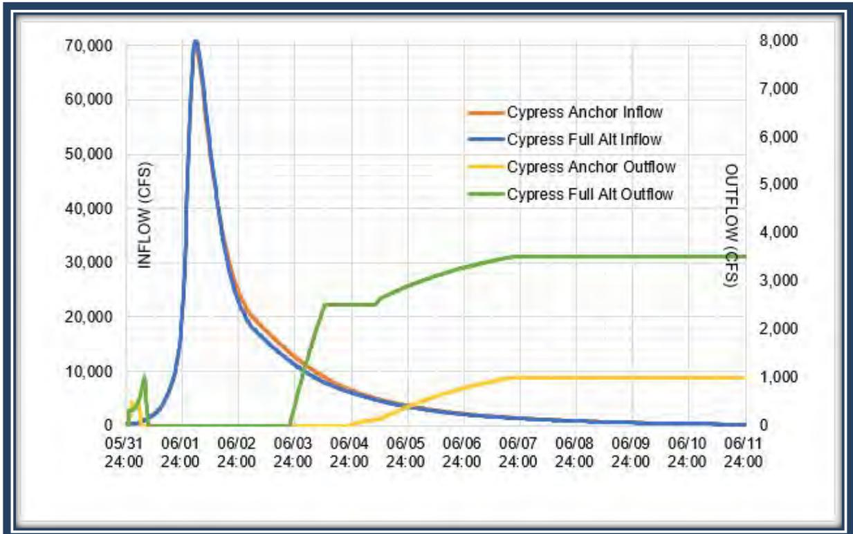
Figure 67. Hydrograph Showing Effect of Alt Plan 2 on Barker Reservoir Inflows and Outflows
