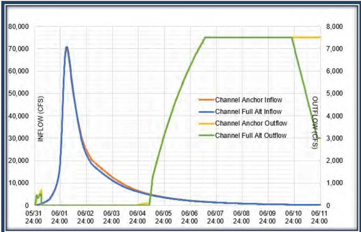
Figure 69. Hydrograph Showing Effect of Alt Plan 6 on Barker Reservoir Inflows and Outflows
