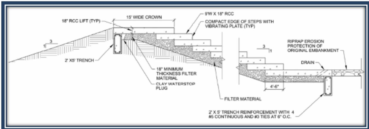
Figure 78. Typical Cross-Section for Stepped Roller Compacted Concrete
