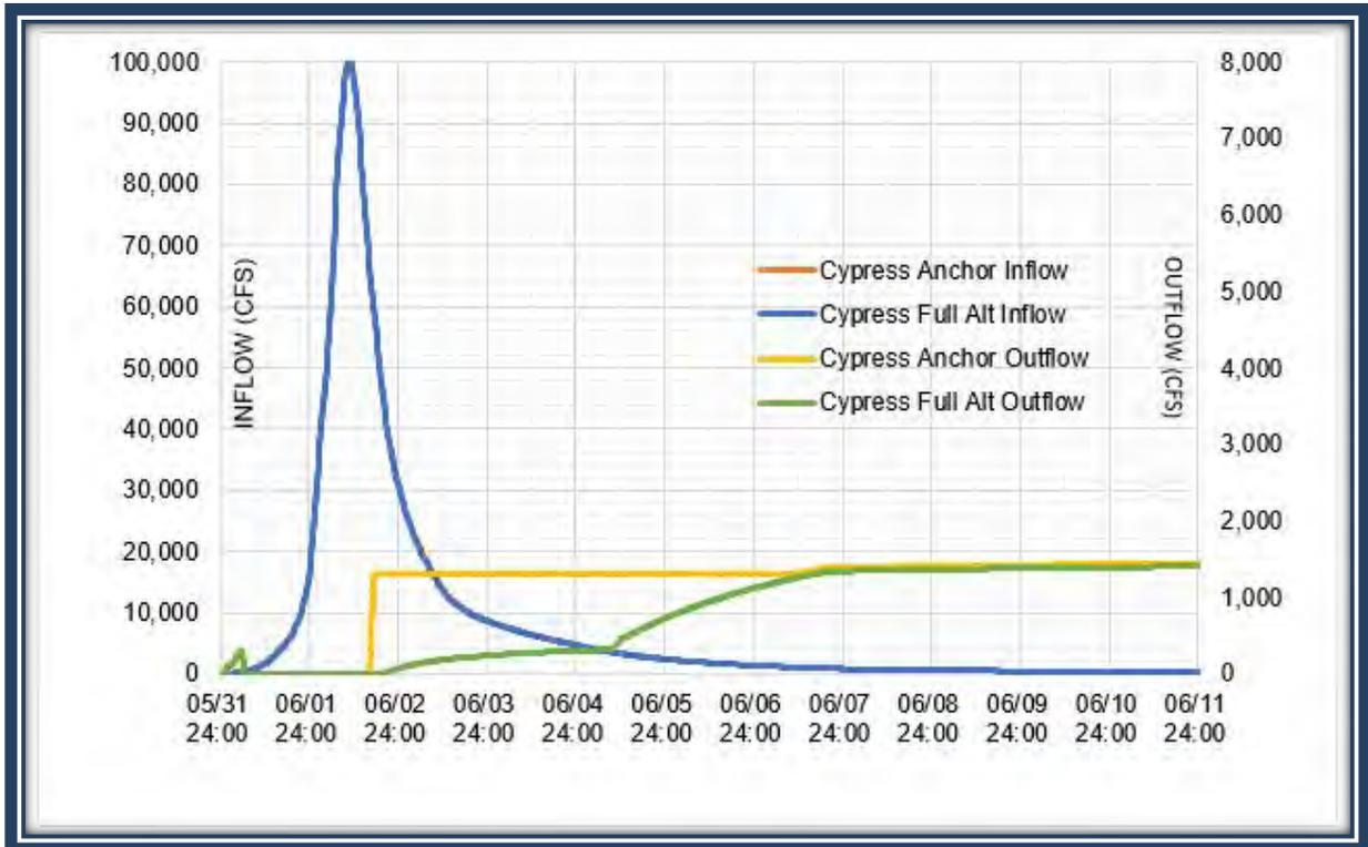
Figure 66. Hydrograph Showing Effect of Alt Plan 2 on Addicks Reservoir Inflows and Outflows
