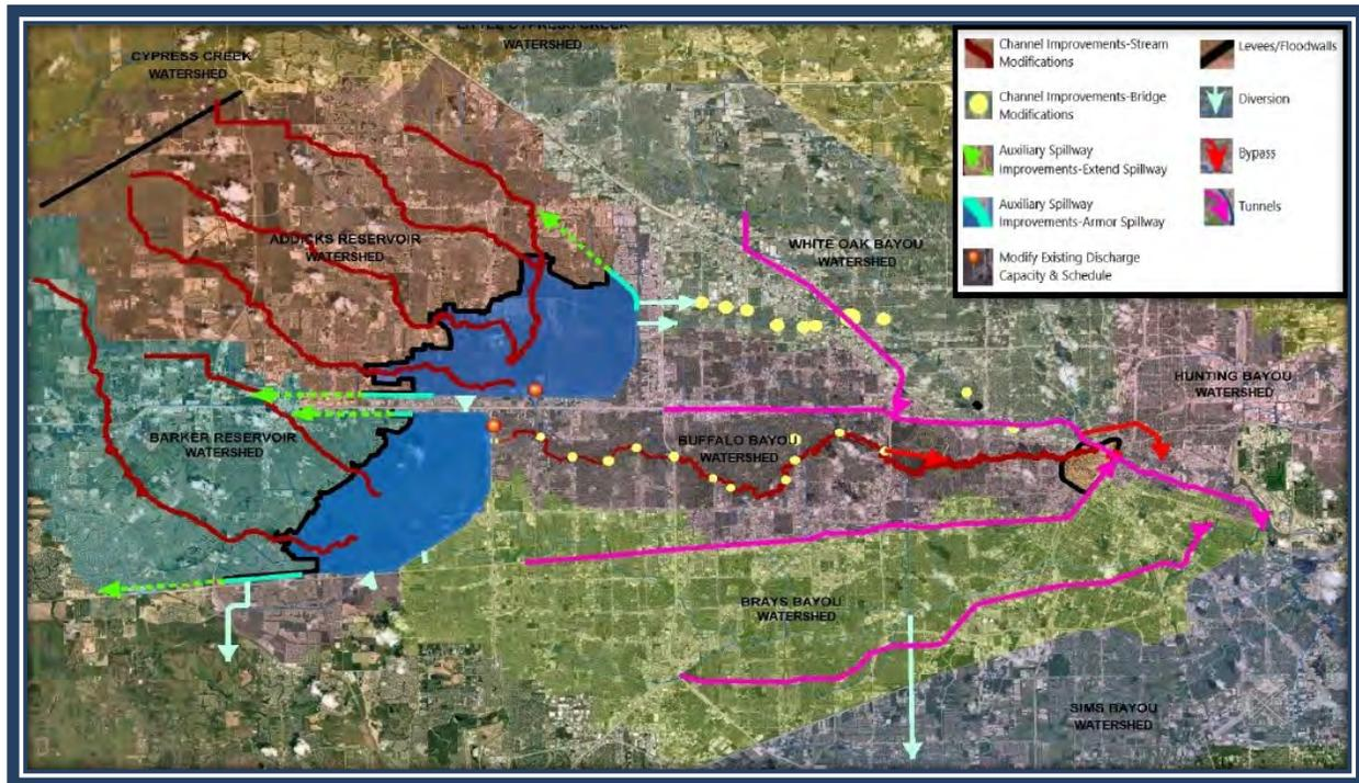
Figure 29. Structural Measures to Increase Conveyance out of the System
