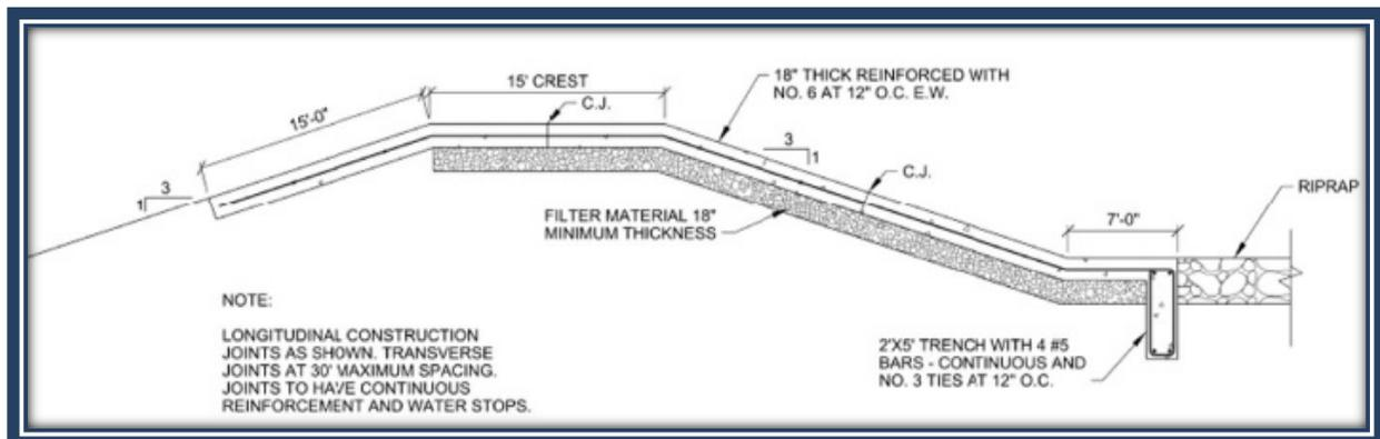
**Figure 74. Example of Reinforced Concrete Slabs**
