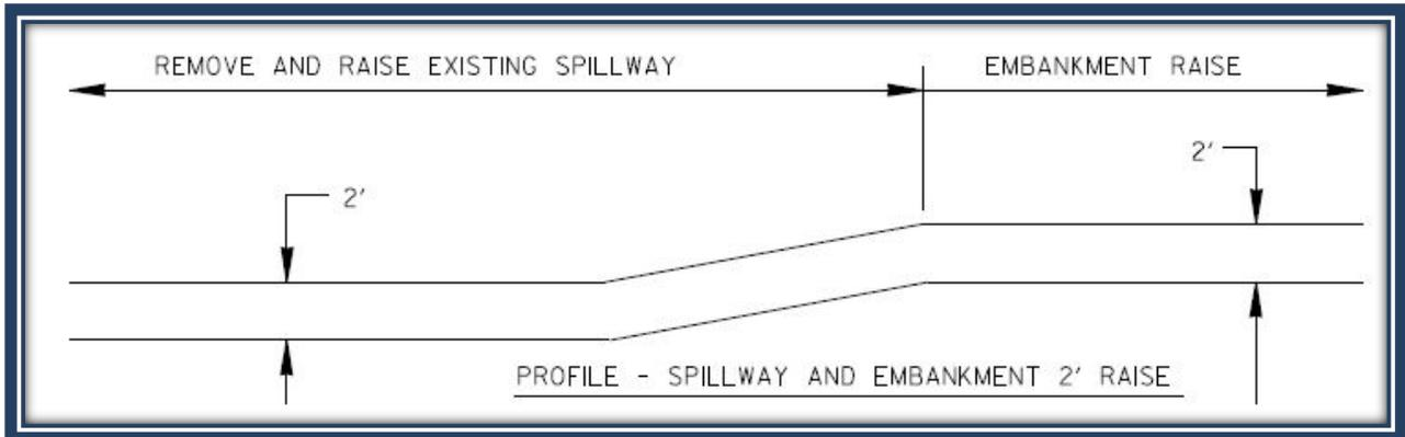
Figure 40. Profile – Spillway and Embankment Raise
