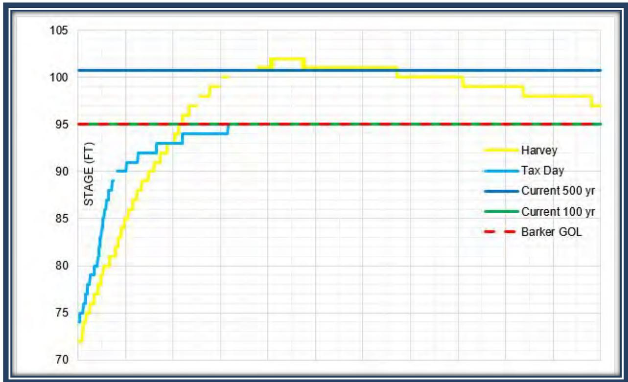
**Figure 2. Observed Elevation of Hurricane Harvey at Barker Dam**
