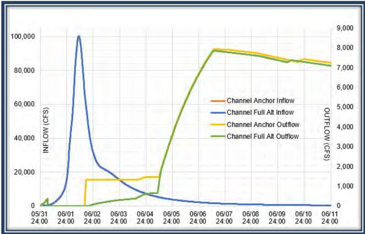
Figure 68. Hydrograph Showing Effect of Alt Plan 6 on Addicks Reservoir Inflows and Outflows
