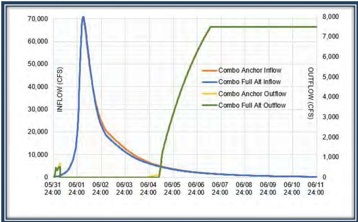
Figure 71. Hydrograph Showing Effect of Alt Plan 8 on Barker Reservoir Inflows and Outflows
