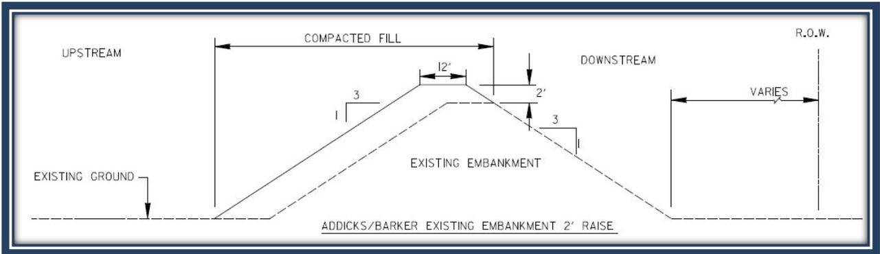
Figure 39. Typical Embankment Raise
