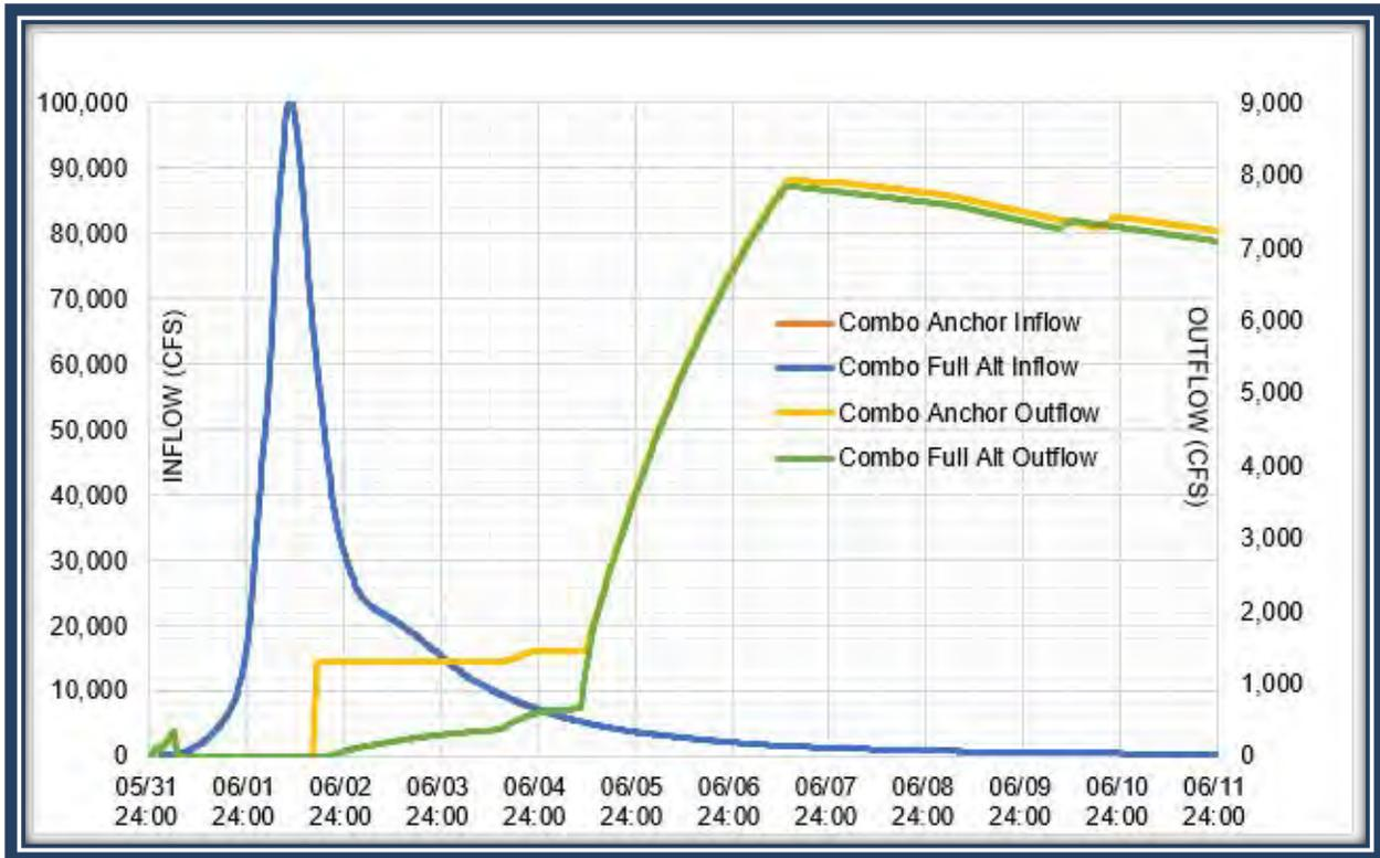
Figure 70. Hydrograph Showing Effect of Alt Plan 8 on Addicks Reservoir Inflows and Outflows
