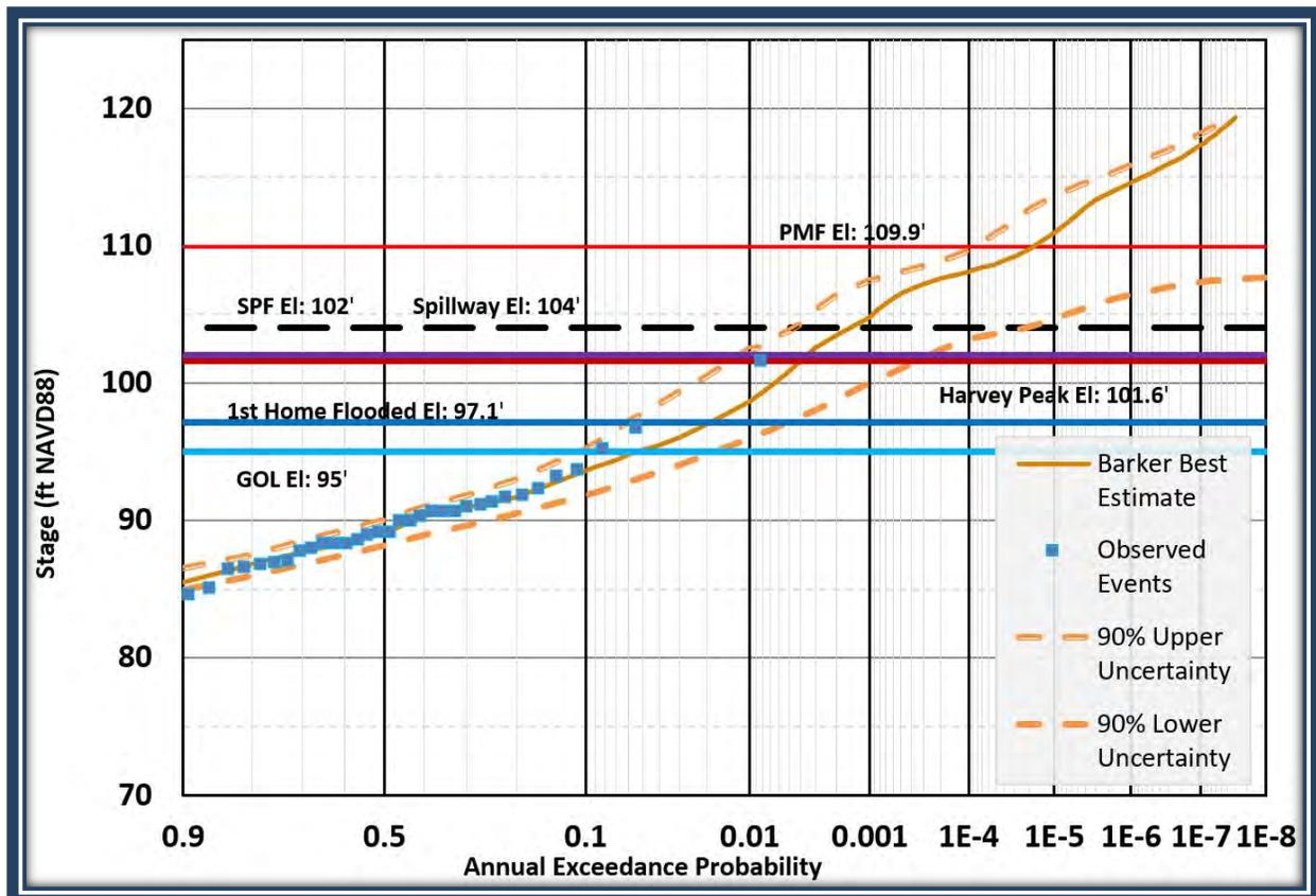
Figure 52. Barker Pool Frequency Curve (USACE 2020)
