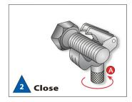
Turn handle (**A**) to lower floating blades into grooves of thread and tighten by hand only.
