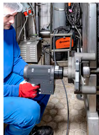
Image above: alkitronic® EFCip-SG in operation on a plate heat exchanger.
