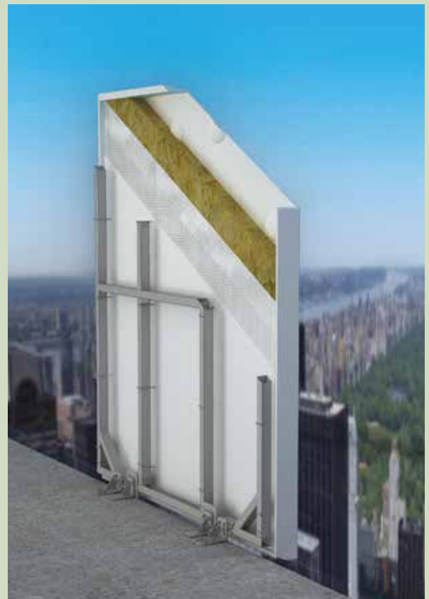
Insulated GRC Shell Panel Detail
