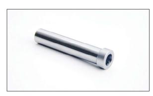
**DESCRIPTION:** KEB Tool Sleeve Holders are manufactured from an aircraft quality alloy steel and heat treated to 28 Rc for greater wear ability. Designed for use on all CNC or manual turning and boring operations.
