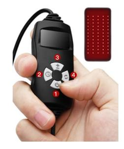
8. To select all LEDS on together select "ALL. To select redlight ONLY Start with the "ALL" view and press button 4 to view 660. Only the redlight is on. Press it again to view 850 now the infra redlights, only, are on. (Infra-red light is invisible so the pad will not show light.
