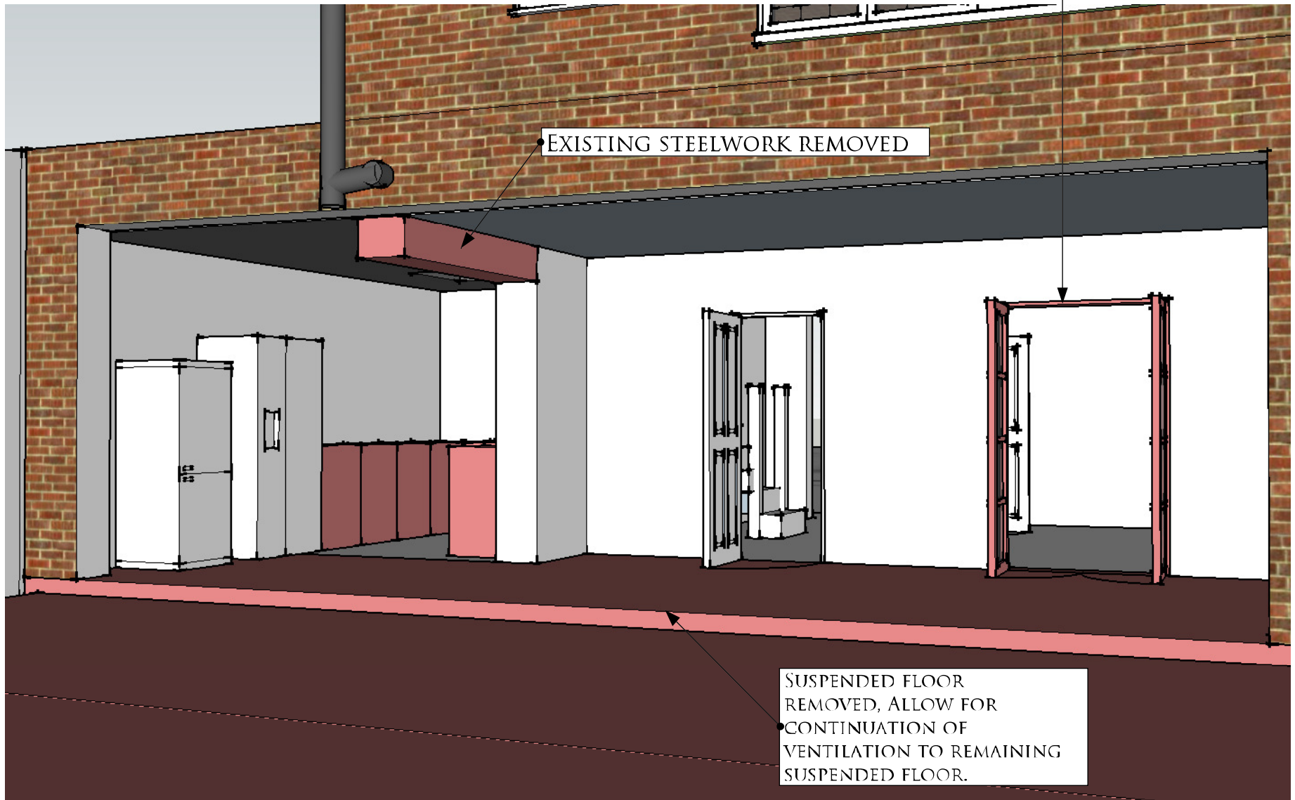
PERSPECTIVE REAR ELEVATION WITH PARTIAL DEMOLITION
