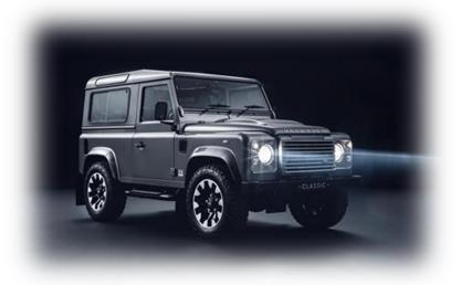
The Defender Classic Works Upgrade Kit includes all of the wheel, brake and suspension elements in addition to new performance-rated tyres and an engine upgrade which delivers an extra 40PS – total output of 162PS and 463Nm torque. Top speed is increased to 106mph.
