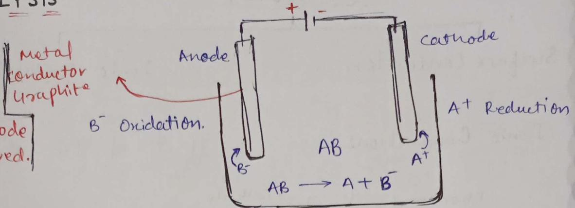
The process of chemical decomposition of an electrolytes by the passing of electricity is called Electrolysis & the cell are called Electrolytic cell.
