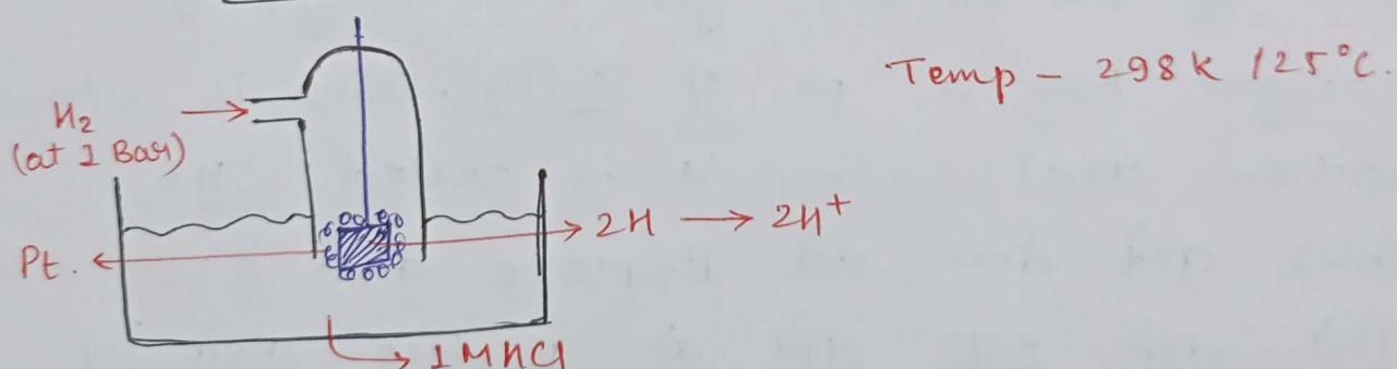
→ when standard hydrogen consists of a platinum electrode which is an anode electrode, which is dipped in acidic solution of 1M and temp 298 K and 1 atm pressure.
