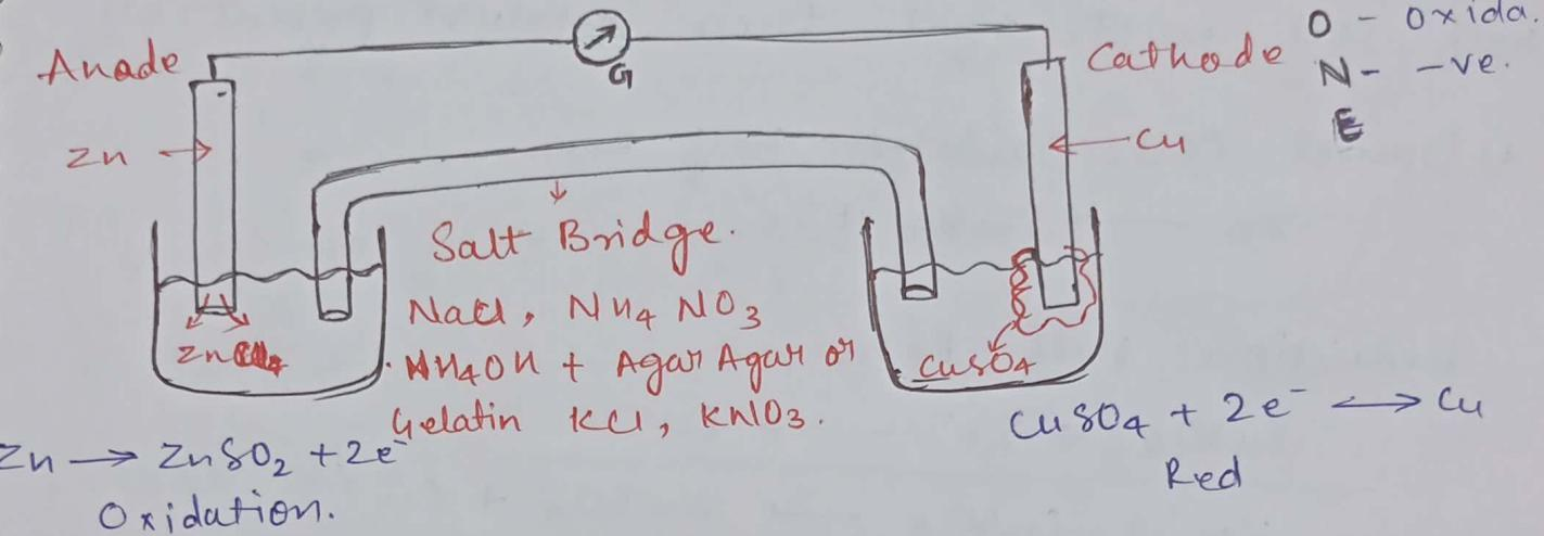
It is also called Galvanic cell two half cells are separated by each other by SALT BRIDGE.
