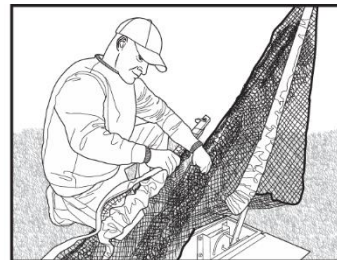
Put Poles down in the reverse sequence that was used to assemble the Unit. Remember to lift pole up in the Bracket before releasing Push Pin
