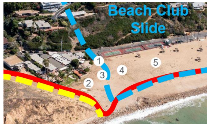
Remove earth to relieve pressure in PBC
