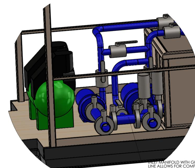
INLET MANIFOLD WITH GUT LINE ALLOWS FOR COMPLETE WATER TRANSFER IN ANY DIRECTION EASY PRIME SYSTEM WITH EITHER FRESH OR RE-CIRCULATED WATER
