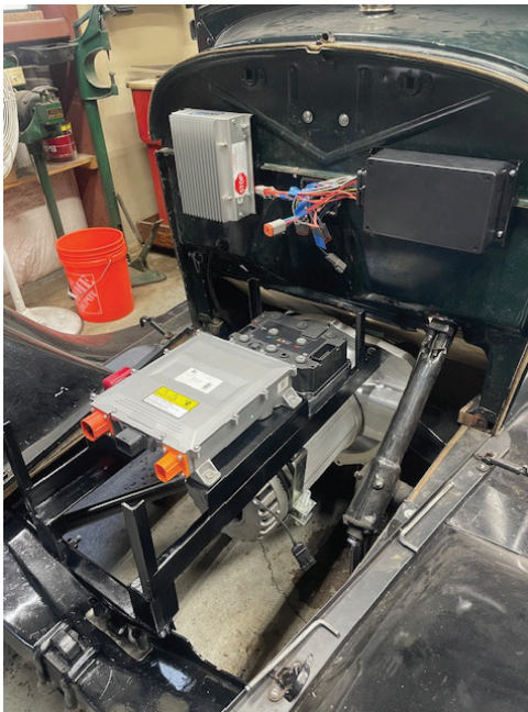
Battery charger and controllers installed using Dennis’ framework, which also acts as the front motor mount.
