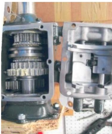
Ray ordered a Mitchell Synchronized transmission with a #3 ratio. The #3 ratio is synchronized in reverse, low and second gear. As things are lately with the supply chain, it took a while to get to him. He ordered it in July of 2021 and received it in late
