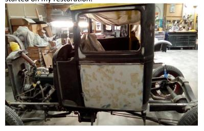
The truck was stripped and Bondo was found everywhere, and some sections the Bondo was so bad, that after sandblasting you could put your hand through it. A lot of fiberglass and repair was done. After repairing all the body work the painting started. New fenders were purchased as the originals were so dented and full of fiberglass. Thus, all redone and painting started.
