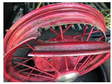
It appears the wheel had water between the rim and inner tube which caused the wheel to rust away in the center. With us running on nearly 100-year-old wheels a close inspection this fall may reveal some interior rust.
