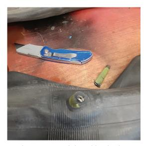
Then, I trimmed the rubber back to within 1/8" of the tube and pulled out the remaining portion of the stem.
