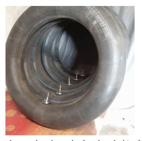
After about an hour's worth of work and a bit of patience, all five valve stems went in with no problems. All that was left was to air check them and put the tubes back in the corner of the garage for a week or two to watch for leaks.
