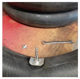
And lastly, I attached the bridge washer and the lock nut.
