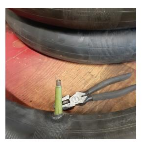
Next, I deflated the tubes and cut off the rubber stems, cutting through the rubber with a razor knife and then cutting the brass core with a pair of side cutters.
