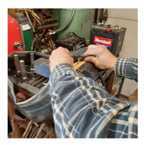
I then lined up the hole in the tube and stretched the tube over the valve stem.
