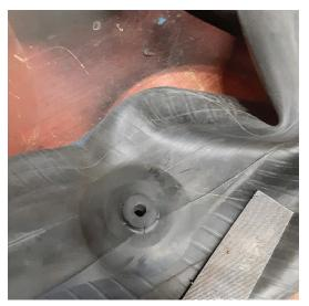
Using a new blade, I trimmed the remaining rubber as flat as possible.
