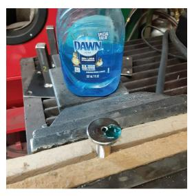
Next came installing the new metal stems. I clamped the new stem in the vise with a couple of pieces of wood to protect it and lubricated it with dish soap.
