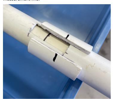
I drilled a hole through both pipes and inserted a cotter pin to keep it all together when stored.
