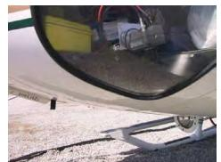
Figure 5. Digital video camera typical mounting location.
