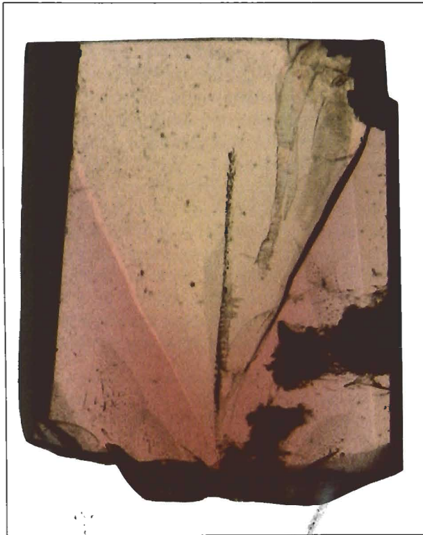
Figure 8. A section cut parallel to the c -axis through a red beryl crystal. Here the width of the light-colored, triangular, central zone decreases from the upper end of the crystal to the bottom (where an included bixbyite grain would most likely be located if it were present). The crystal is about 0.5 cm long. Transmitted light, partial shadowing, magnified 15 \times . Photo by John Koivula.
