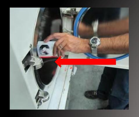
Open the door and spread the contents of one packet of Chamber Brite™ in a straight even line along the bottom of the chamber, from back to front. Do not leave a pile of Chamber Brite in one spot.
