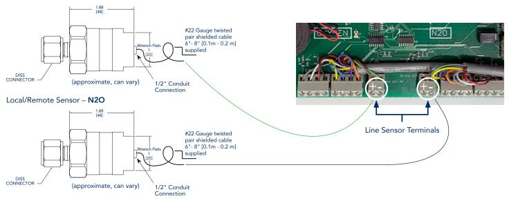
Identify the appropriate gas sensor wire and connect it into the appropriate terminal, taking attention to the polarity. Connect power to Manifold and test that the pressure is being read at the zone valve box. This can be done by closing a valve and bleeding downstream.
