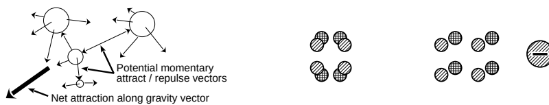
Figure 13. Left, object in 3-D space pulled away from or in shear to the overall gravitational force vector; polarization: center, electrically neutral object with uniform proton-electron count; right, like charges (electrons) move away from strong external charge while opposite charges (protons) move closer.
