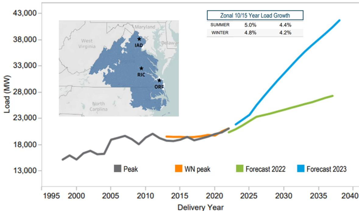
The data center load growth rate (currently concentrating in areas of northern Virginia) continues to increase. FirstEnergy’s APS zone (just north of Virginia) is also experiencing data center load development, driving high flows within the northern Virginia transmission system, into the data center concentrated load pocket. The 2027 and 2027/28 study cases summer zonal load for Dominion and First Energy is provided in **Table 1**.
