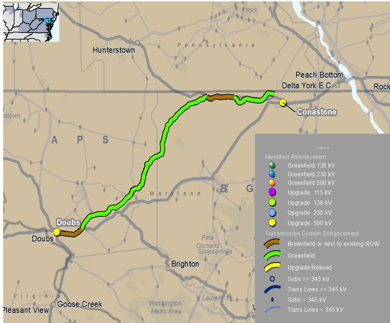
Proposal 837 by FirstEnergy builds a new Hunterstown-Carroll 230 kV line in addition to rebuilding the existing 115/138 kV corridor as double circuit using 230 kV construction standards.
