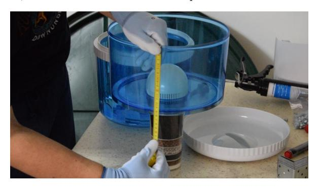
Take this dimension and measure it down inside the barrel – starting at the holes you drilled earlier.
