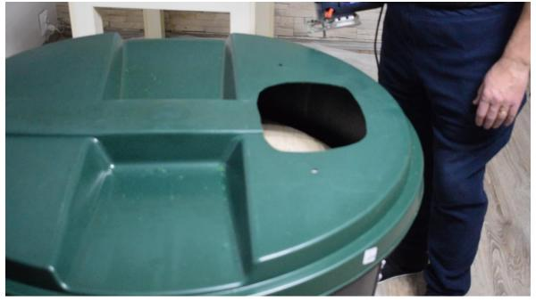
One more thing to do here: Drill two holes in the lid for the in/out tubes going to/from the dehumidifier. I drilled them to the left and right of the dehumidifier opening above.
