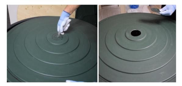
Due to the fact that the lid might not have the same diameter as the inside of the barrel, brings us to the next operation. Fitting the lid inside the barrel – onto the lower supports.
