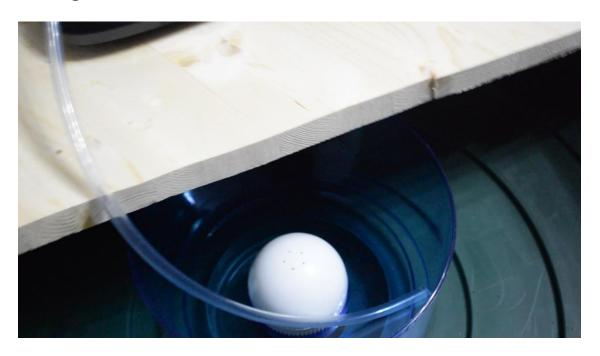
**Step 14.**Place the dehumidifier inside the barrel and fix it on its support.
