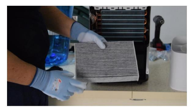
You might need to cut and adjust the cabin air filter to fit in the dehumidifier.
