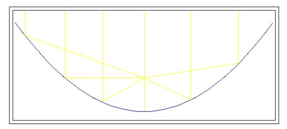
Mathematically, a parabola is defined as a set of points that are the same distance from both a point (called the focus) and a straight line (called the directrix).
