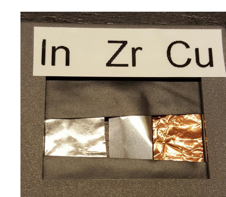
Colour x-ray test object, made of 3 elements, pure samples
