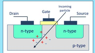
Fig. 4: interaction of radiations with electronics.
