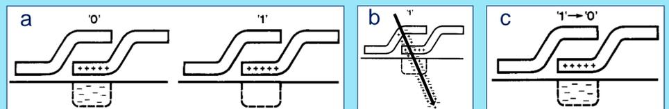
Fig. 5: soft error caused by a single particle in a DRAM. [1] The memory state of a DRAM depends on the charge of a capacitor (fig. 5a). The free charges generated by the incoming particle (fig. 5b) can cause the transition between two memory states (fig. 5c).
