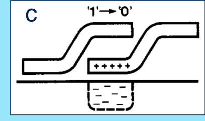
Fig.5: soft error caused by a single particle in a DRAM. [1] The memory state of a DRAM depends on the charge of a capacitor (fig. 5a). The free charges generated by the incoming particle (fig.5b) can cause the transition between two memory states (fig.5c).
