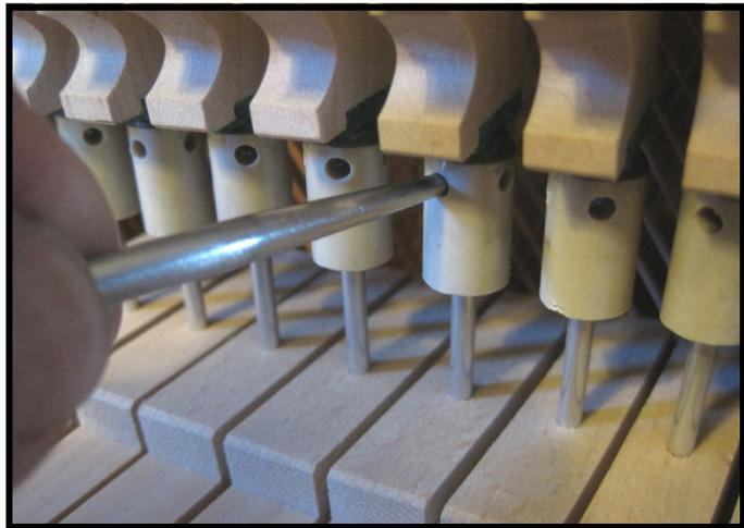
Pianos go "out of regulation" over time because of the fact that for every important adjustment which is made there is a corresponding felt cushion which buffers the contact points between the parts of the action. These felt cushions become compacted with age and use, and the various regulating adjustments made in the factory need to be redone in order to compensate.
