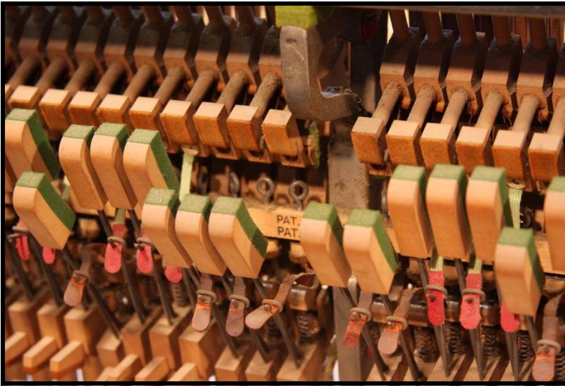
One example of parts which commonly needs to be replaced on a vintage upright piano is the bridle straps, shown in the photo to the left. These straps are essential for holding the bottom of the action up when it is removed from the piano for servicing.
