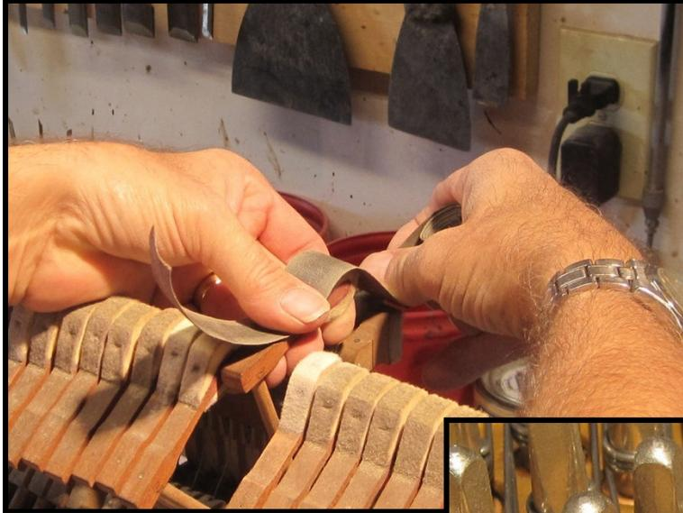
Hammers are being carefully shaped in the photo to the left to remove cut marks caused by strings. This will result in an improvement to the tone of the piano. In cases of severe wear, replacement of the hammers may be a better option.
