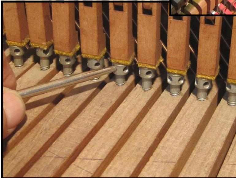
An unwanted quantity in the operation of the piano action is "lost motion," or wasted energy. In the photo to the left, lost motion is being taken up by the careful regulation of brass capstans.
