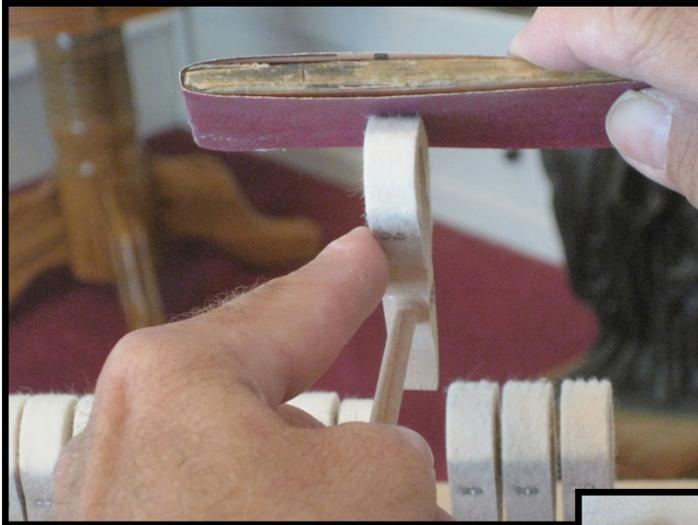
An old, worn-out set of hammers may very well need attention in a piano that has been played hard over the years. Careful reshaping of the hammerheads is sometimes possible, as is being done in the photo to the left. At other times where the old hammers are badly worn, the installation of a new set of hammers is necessary.
