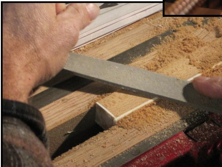
Original ivory in good condition on an older grand piano is a definite plus. A few chipped keys may oftentimes be replaced or repaired. In cases where the old keys are badly worn, however, installing a new set of keytops (shown being fitted to the keysticks) will benefit the appearance of the piano.
