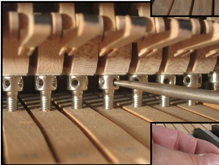
Hammers are adjusted so that they are perfectly level from one end of the action to the other. Here, the height of the hammers is regulated by precise adjustment of the appropriate brass capstans.
