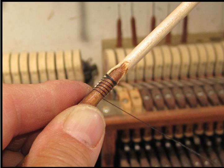
One example of a part which might need to be replaced or repaired on a grand piano would be that of a broken hammer shank. Each shank connects to a hammer, and as such is subject to a great deal of stress and occasional breakage. In the photo left, a new section of shank is spliced to the bottom of an old shank which had broken.
