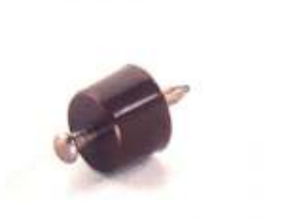
PLASTIC SHELF SUPPORT WITH LOOSE NAIL
